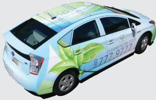
A vehicle is wrapped with a design printed onto special 3M vinyl which is then laminated and applied (“wrapped”)
